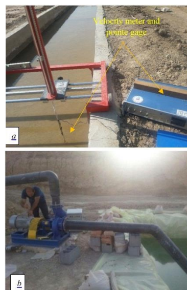
Fig. 4. a) Velocity meter and pointer gauge b) A centrifugal pump placed in field laboratory
