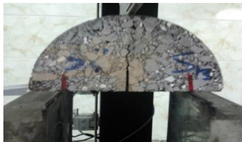
Fig. 4. Fracture path observed for the SCB specimen after fracture test
