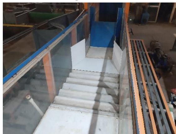
Fig. 5. A view of corrugated bed and expansion
