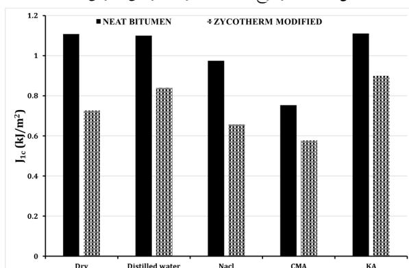
Fig. 11. Critical energy release rate ( $J_c$ ) values
