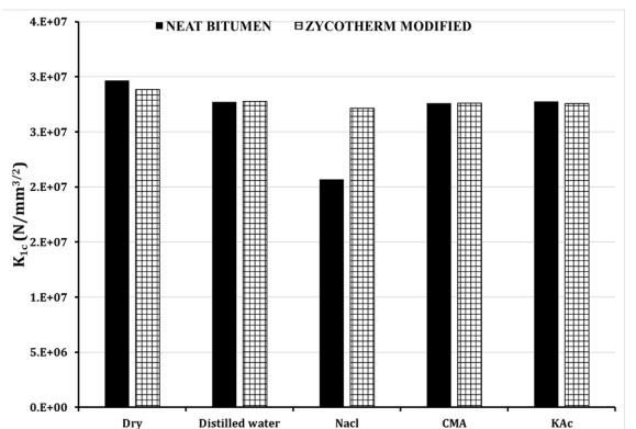
Fig. 10. Fracture toughness of asphalt mixtures at low temperature
