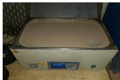
Fig. 2. Asphalt mixture conditioning in CMA
