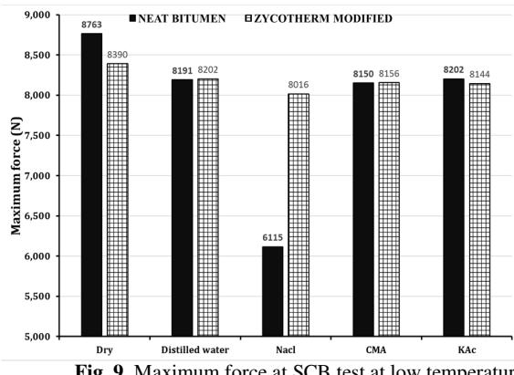
Fig. 9. Maximum force at SCB test at low temperature
