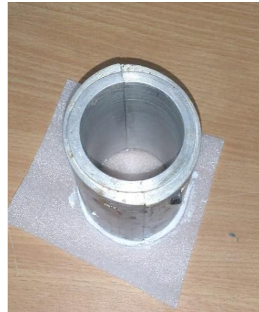
Fig. 3. Curing mold of frozen soil specimens.
