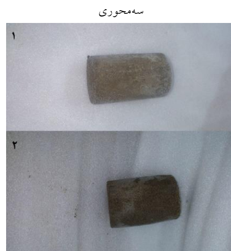
Fig. 7. Frozen soil specimens: (1) before test, (2) after test.
