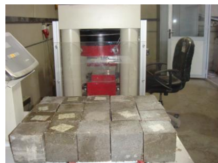
Fig. 2. Concrete specimens and test machine
