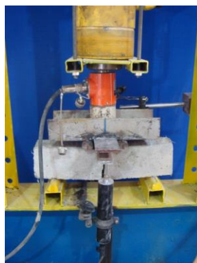
Fig. 4. Flexural test machine and specimens
