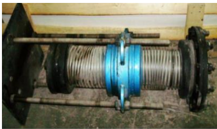
Fig. 7. Primary sample of contractable viscous dashpot
