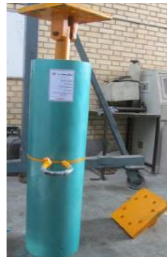
Fig.9. A Full-scale contractable viscous dashpot
