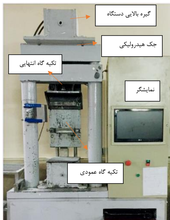
Fig. 3. Single-lap shear test setup
