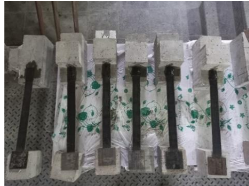
Fig. 7. Strengthening of specimens
