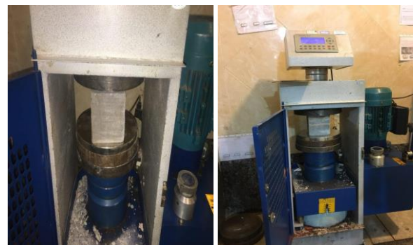
Fig. 3. Compressive strength test on RPC samples
