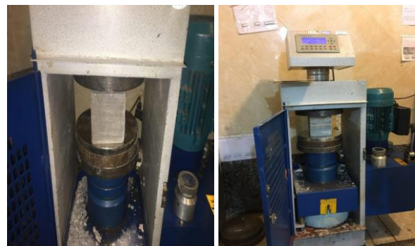
Fig. 3. Compressive strength test on RPC samples
