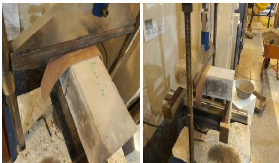
Fig. 4. Bending strength test on RPC concrete beam
