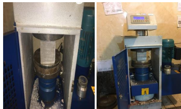
Fig. 3. Compressive strength test on RPC samples
