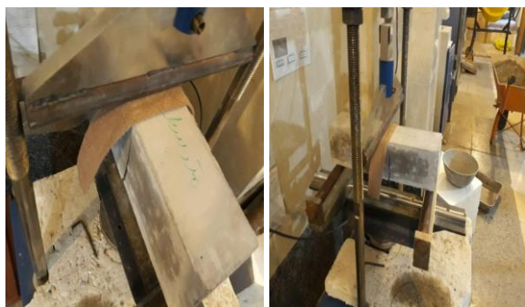
Fig. 4. Bending strength test on RPC concrete beam
