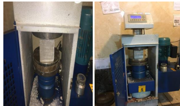
Fig. 3. Compressive strength test on RPC samples
