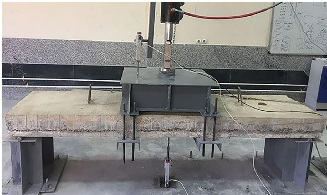
Fig. 5. Details of the flexural test setup of experimental specimens
