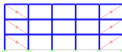
Fig 3. 3-stories bending frame with viscous damper
