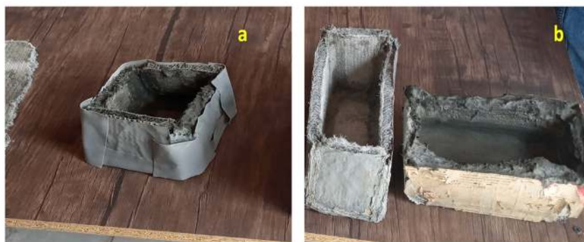
Fig. 8. Product made of fabric concrete made with polymer casting technology (sample A related to the product made on the basis of geo-membrane layer and sample B related to the product made based on casting)
