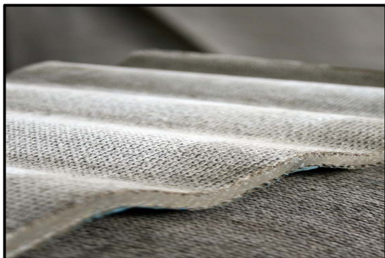
Fig. 1. Scheme of concrete canvas structure
