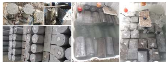
Fig. 4. Manufacturing, sampling, and curing processes of specimens
