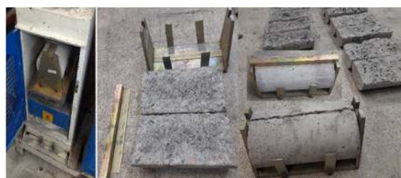
Fig. 7. Process and tools for tensile testing
