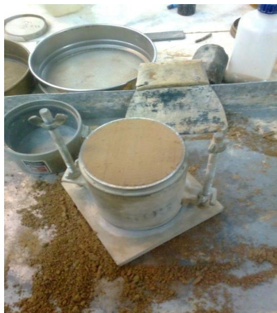
Fig 3. The sample preparations and placing it in the special frame of the Hole Erosion Test.
