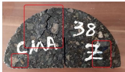
Fig. 6. Samples submerged in CMA
