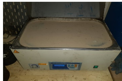
Fig. 2. Asphalt mixture conditioning in CMA
