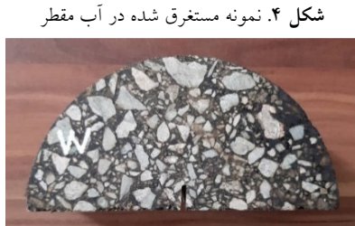
Fig. 4. Sample submerged in distilled water
