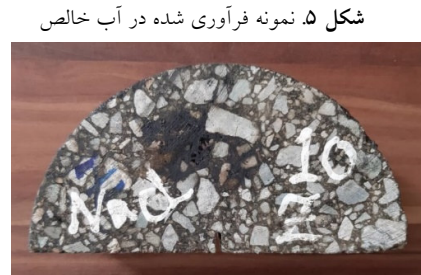
Fig. 5. Sample submerged in NaCl
