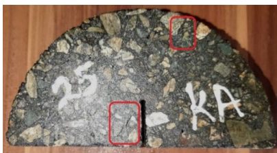
Fig. 7. Sample submerged in KAc
