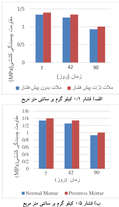
Fig. 6. The results of the pull-off tests on mortars under different prestresses
