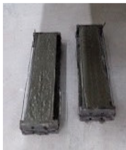
Fig. 2. The prismatic specimen of shrinkage
