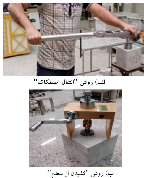
Fig. 3. Evaluation of the compressive strength of mortars
