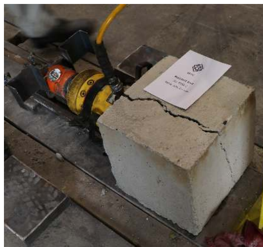
Fig. 9. Picture of split concrete (P25S-2) after test
