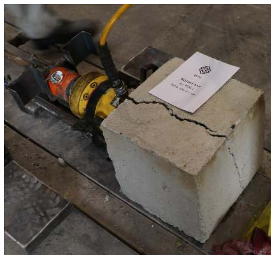
Fig. 9. Picture of split concrete (P25S-2) after test
