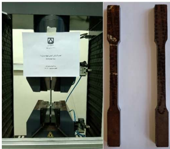
Fig. 3. Universal testing specimens and the diagram
