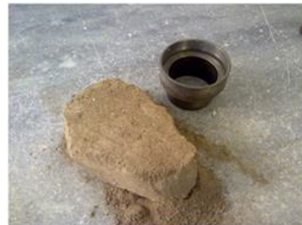
Fig. 5. Cut piece from obtained in-situ intact sample
