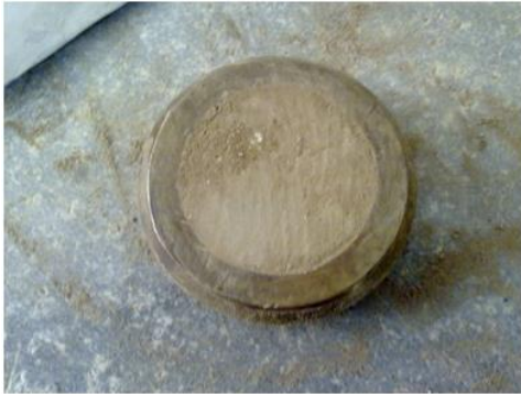
Fig 7. Transferring the intact specimen into the ring of the consolidation apparatus.
