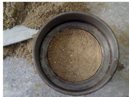
Fig. 6. Taking an intact sample with a sampler
