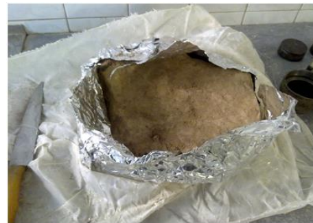
Fig. 4. In-site intact block sample
