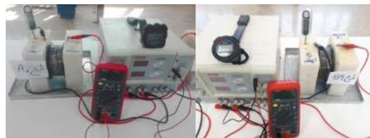
Fig 3. RCPT test according to ASTM C1202 standard
