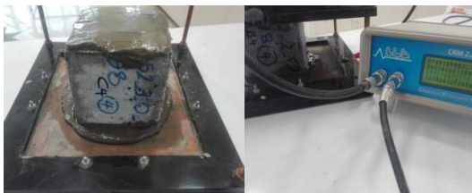
Fig. 4. Electrical resistance test
