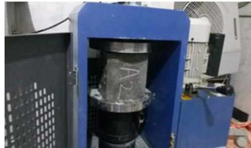
Fig. 5. Compressive strength test according to ASTM C 109 standard
