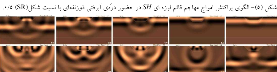
Fig. 5. Snapshots for a trapezoidal-shaped sedimentary valley with SR=0.5 subjected to the SH -waves with the incident angle of \theta = 0^\circ .
