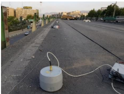
Fig. 4. Molecular-electronic seismometer sensors while gathering vibration data
