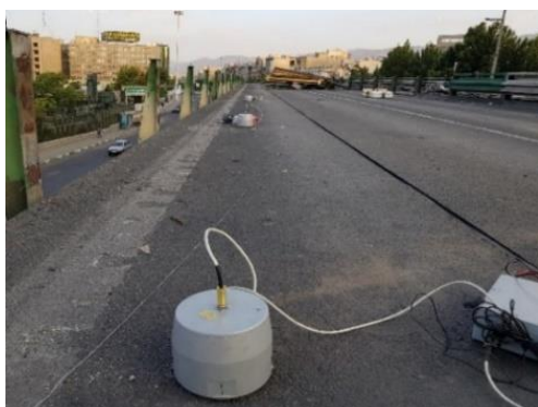
Fig. 4. Molecular-electronic seismometer sensors while gathering vibration data
