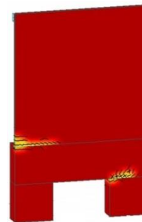
Fig. 15. Distribution of tensile strength and final cracking pattern- Lf=3.5m
