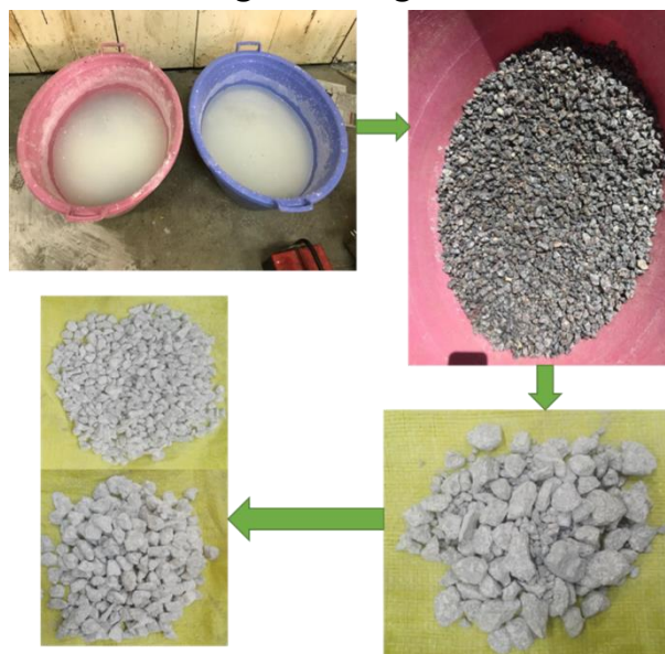
Fig. 1. RCA materials. a) untreated b) treated with liquid Hydrated Lime
