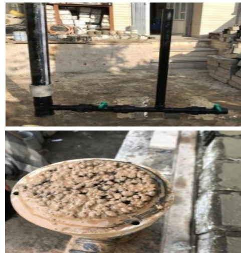
Fig. 2. Constant head device (top), permeable sample after clogging test (bottom)
