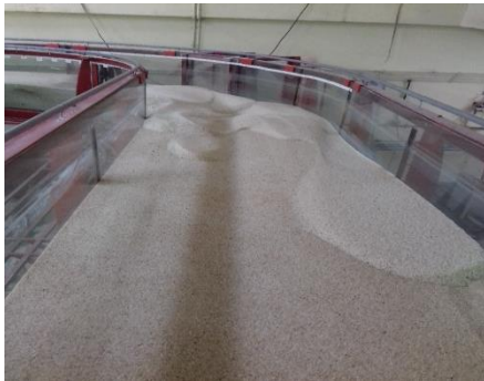
Fig. 9. An instance of bed at the downstream straight end, (D-V)I120 experiment
