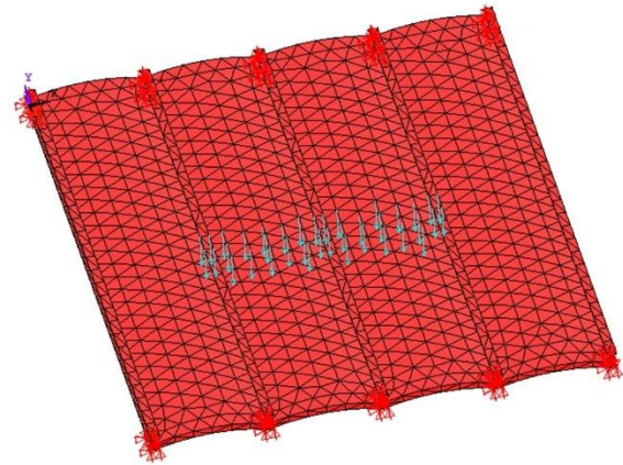
Fig. 11. The modelled jack arch roof for calibration
