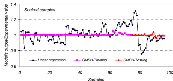
Fig. 9. Variation of models output ratio to real value for soaked samples
