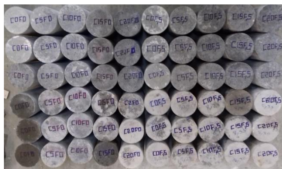
Fig. 3. Specimens for indirect tensile test and compressive strength test
