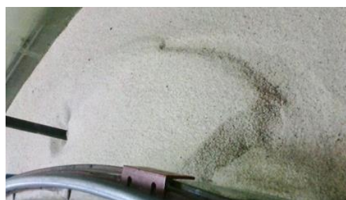
Fig. 5. The view of sedimentary deposit formation on the inner bank
