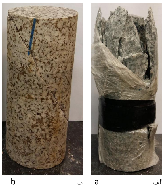
Fig. 7. Failure mode of specimens: (a) kept at room temperature (b) heated to 800°
