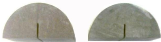
Fig. 8. SCB specimens for laboratory tests
