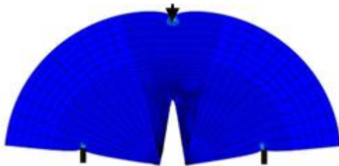
Fig. 11. Fracture path for crack after loading
