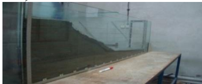
Fig. 9. Completed rupture of saturated unreinforced slope
