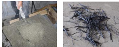
Fig 5. PPS Fiber and FRC concrete
