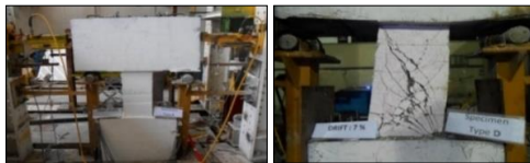
Fig 8. Specimen D, before and after loading
