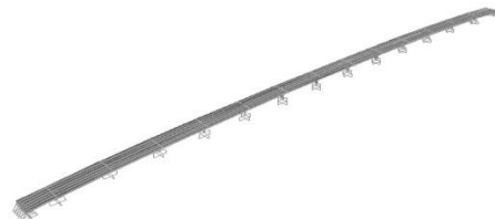
Fig. 5. SAP2000 model of the College Bridge
